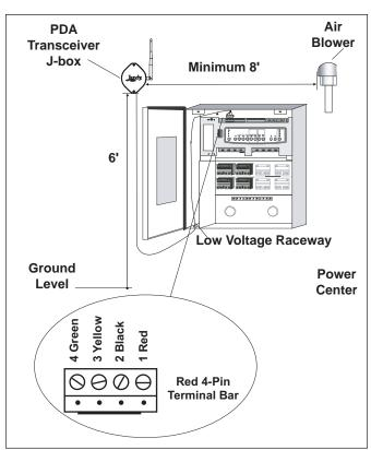
Figure 18. Outdoor Transceiver J-box Installation
